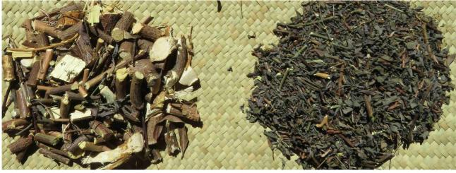
The chipped twigs are 320kg/m<sup>3</sup>, which is a fairly good bulk density for a cooking fuel. The presence of thin stem pieces makes it easy to light and the majority of thicker stem pieces makes it burn longer and hotter. Onces ignited the intensity of the fire can be controlled by adjusting the air inlet of the rocketstove. This fuel could be made available at arround 350 Ar/kg final customers price.
